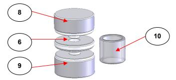
Fig 2. 7mm Pellet Die Assembly Complete
