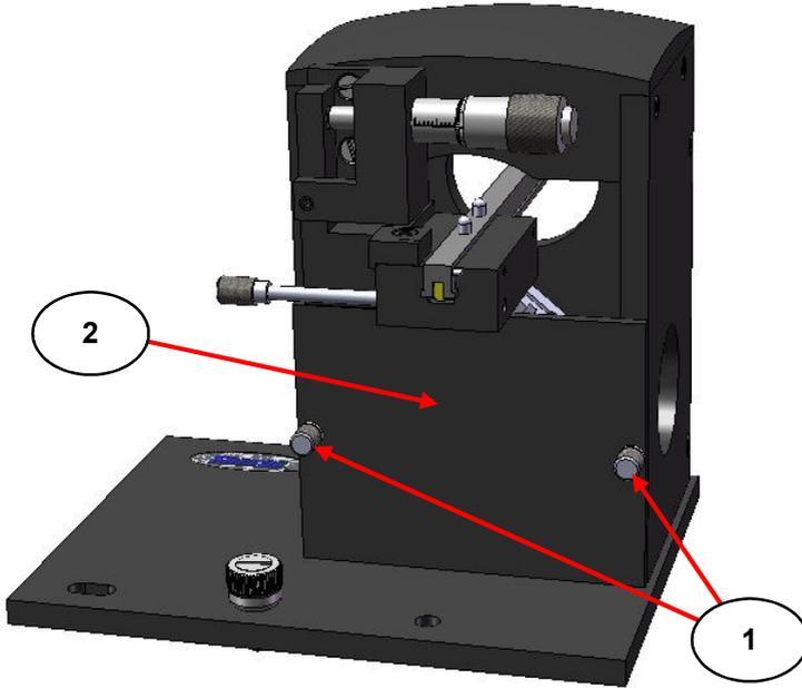
**Fig 1. Front Metal Cover Plate of Minidiff Plus Optical Unit**
