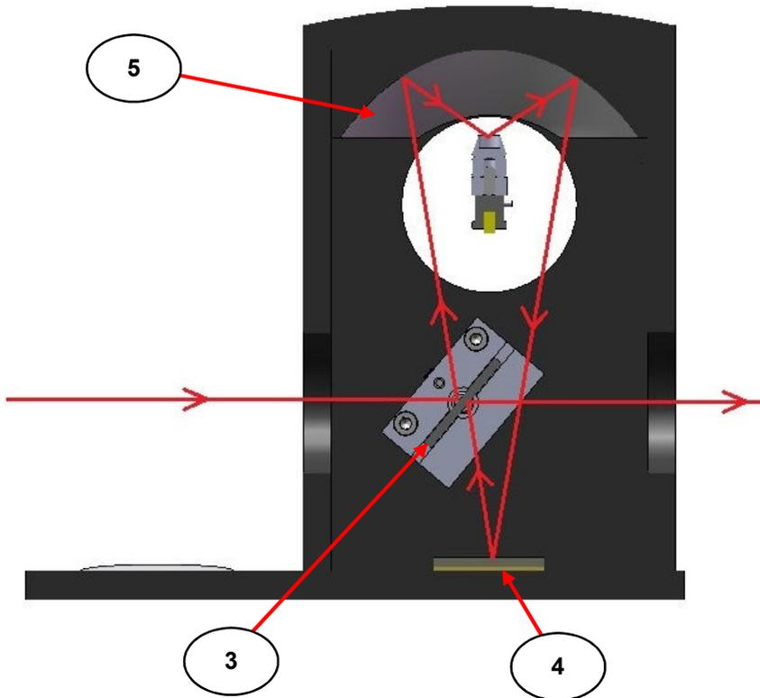
**Fig 10. Beam Pathway Schematic for the Minidiff Plus Diffuse Reflectance Accessory**
