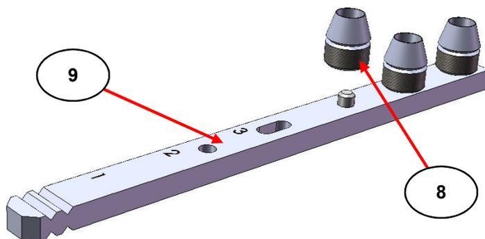
**Fig 6. Fitting of Sample Cup to the Mount Holder Assembly**
