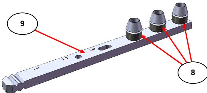
**Fig 5. Minidiff Plus Sample Cups on Mount Holder Assembly**
