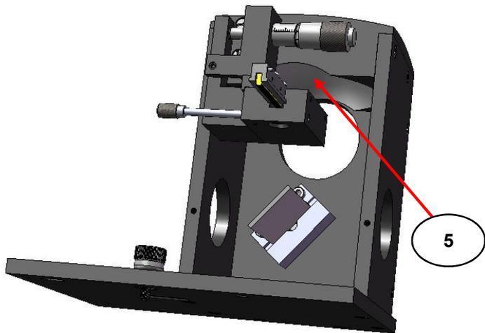
**Fig 3. Minidiff Plus Ellipsoid Mirror Above Sample Position**
