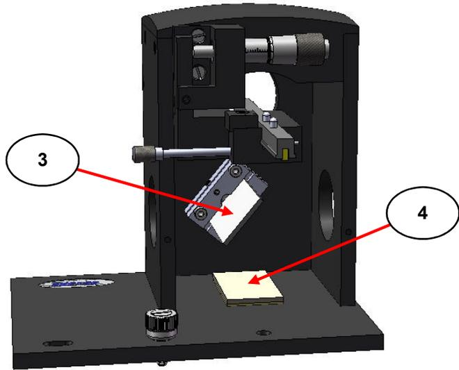
**Fig 2. Minidiff Plus Flat Mirror Assemblies Below Sample Position**
