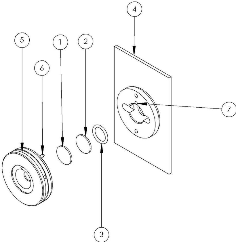
**Fig. 1 – Schematic of Micro Compression Cell Components**
