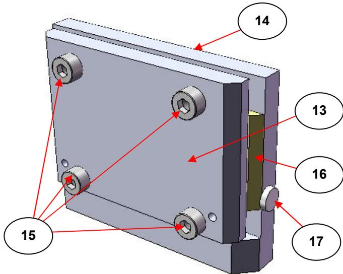
**Fig 3. Solids Holder Assembly with ATR Crystal**
