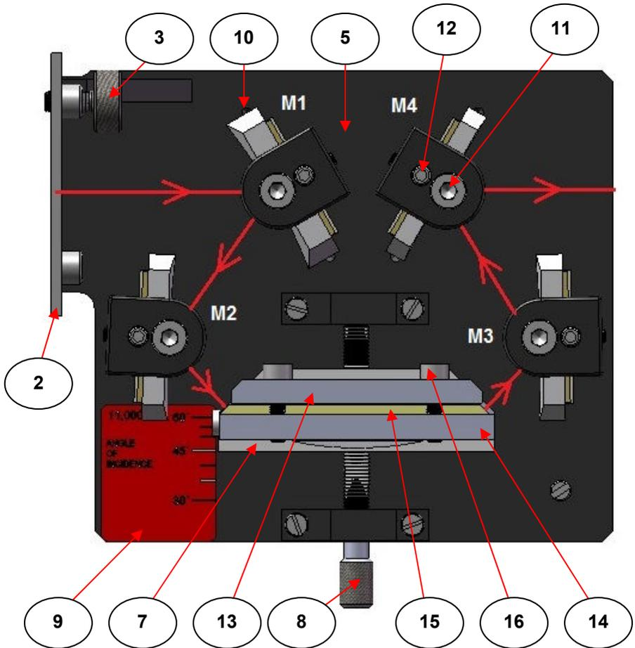
**Fig 8. Optical Path Diagram and Parts Identification for the 25 Reflection Variable Angle ATR**
