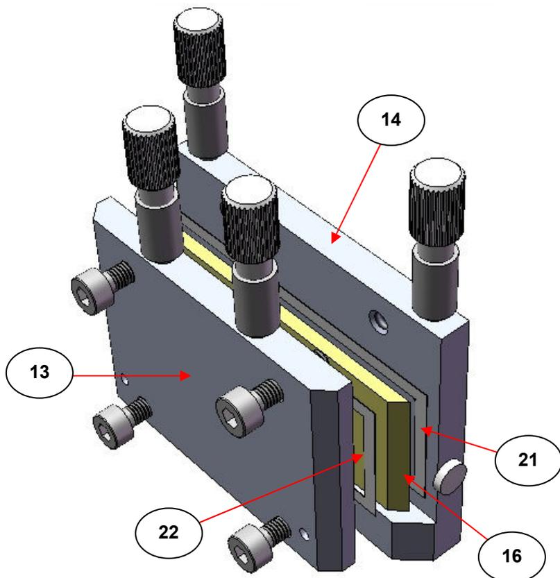
**Fig 7. ATR Crystal with Gaskets for Sample Cavities as Positioned in the Liquids Holder**
