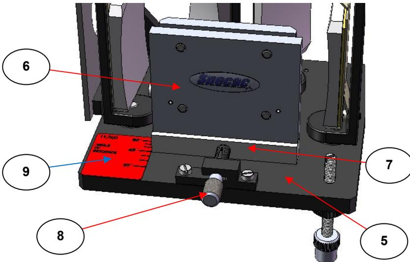
**Fig 2. Translation Stage with Fitted ATR Crystal and Solids Holder Assembly**
