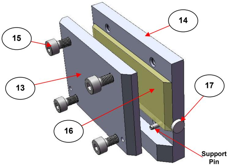
**Fig 4. ATR Crystal as Positioned in the Solids Holder**
