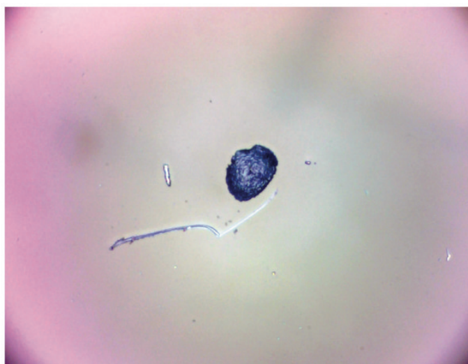
Figure 2: Digital micrograph of an excised contaminant recorded on SurveyIR.
